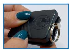
Open the BMW Driver Tag with the help of a flathead screwdriver. Then replace the discharged battery with a new CR2450 battery.
