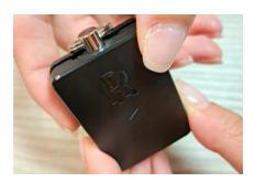
Open the tag with the help of a flathead screwdriver. Then replace the discharged battery with a new CR2450 battery.
